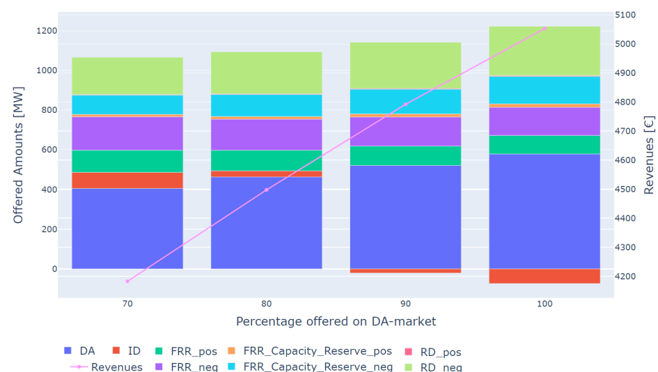
Figure 6. On the x-axis, there is the percentage of the forecast, which could be offered at the day-ahead market (including balancing capacity market); the rest has been traded at intraday markets (including balancing energy and redispatch market). The simulation data are for Zone West, from July to December 2019.
